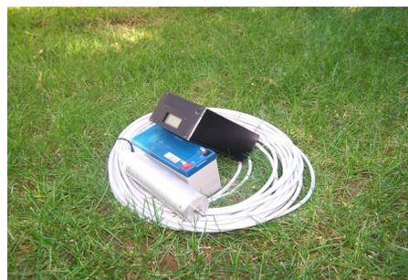
*The SRI32L recorder with the C100 passive sensor*
