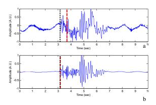
Figure 4: (a) Synthetic seismogram with addition of real seismic noise, (b) Filtered in the Time – Frequency domain signal. The red dashed line is the automatic pick as claculated using the kurtosis criterion and the black dotted line is the actual position of the first break arrival.
