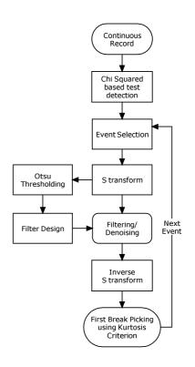
Figure 1: Flow chart of the stages of the proposed method.
