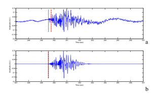
Figure 7: The event selected from (a) the real data and (b) the filtered in the Time – Frequency domain. The red dashed line is the automatic pick as calculated using the kurtosis criterion and the black dotted line is the actual position of the first break arrival.
