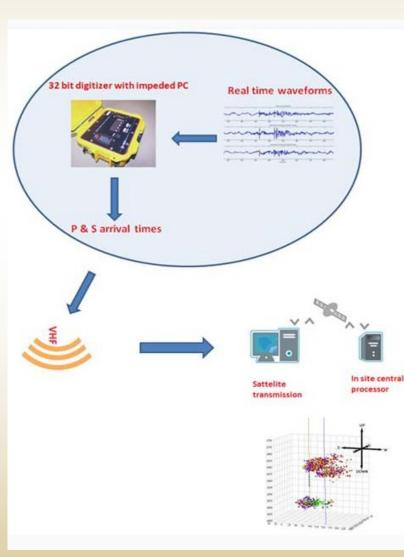
One is based on Wi Fly technology (which is much better than the conventional Wi Fi). The characteristics of this system are: Real time data (full waveform) transmission, Station connections in chains – manual addressing mode, Ability for repeater usage if not clear line of sight, Error correction transmission algorithm, Satellite transmission of the network data in near real time.
