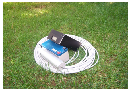
The SRI32L recorder with the C100 passive sensor
