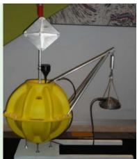
SENSOR: A special designed sensor casing is provided, to support a pressure of 1200 atm. The coupling has been optimised in order to maximise sensitivity.
