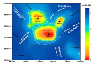
V/V/VS Ratio In the figure to the left, we present another example on how a PST survey revealed clearly the mechanisms controlling a geothermal field
