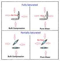
In fully saturated rocks first order intercrack flow may occur only in shear, not in compression. Since the P wave is strongly affected by bulk compression it is less attenuated than
